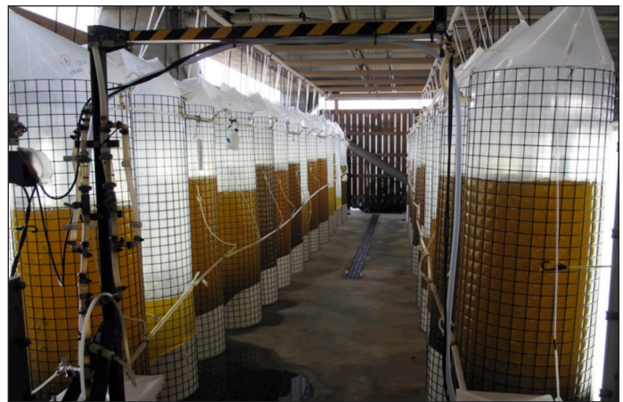
Figure 5. A typical installation of a 28-bag continuous algal bag production system.
