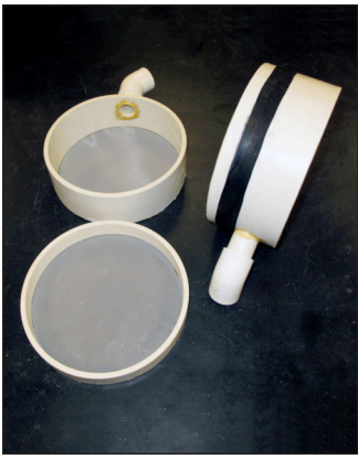
Figure 3. Banjo screens made of 8-inch-diameter thin-walled (sewer) PVC pipe. Screens are made in two pieces (left) to take apart for easy cleaning and held together with a custom rubber band (right). The seawater discharge pipe is made of 1-inch-diameter PVC pipe mounted flush with the screen wall's interior using epoxy resin. A 45-degree PVC elbow is used to connect the screen to the tank's seawater discharge pipe.
